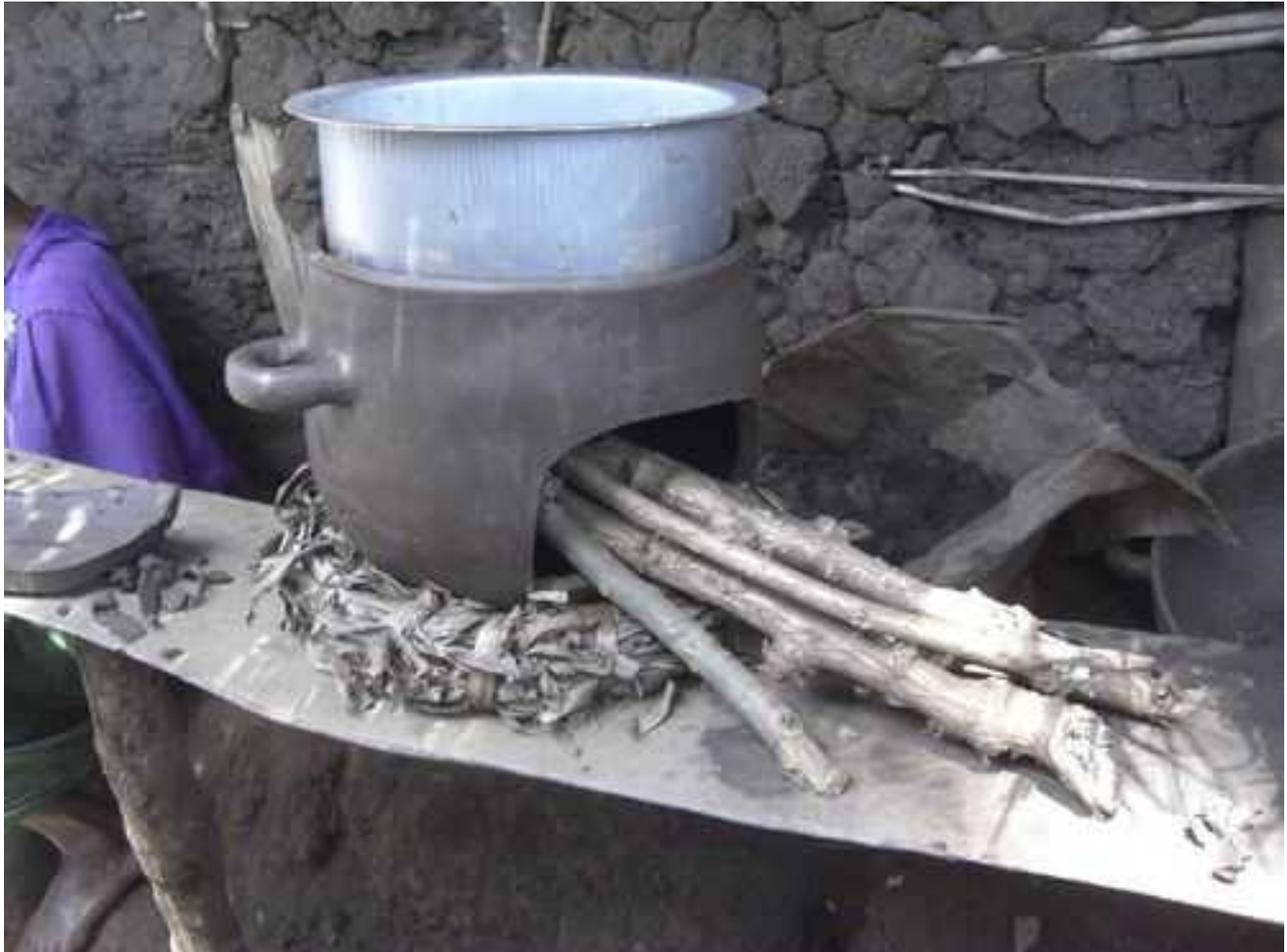
Any clay suitable for making pots should be suitable for making a clay stove. One possible source may be termite or anthill mounds, as often this is fine material dug from deep underground. If necessary crush the clay into dust before adding water.
