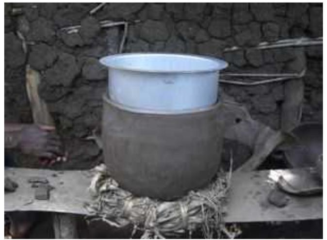
12. Check the pot can now sit inside the stove. There must be a sufficient gap for smoke and flames to escape between the pot and stove. (For an alternative design, place 3 blocks around the top, for larger pots to sit on top of the stove.)
